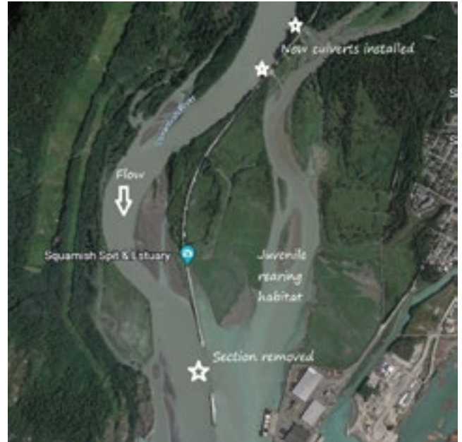
Three hundred metres of the berm in the Squamish River Estuary have been removed, and work is planned for January 2023 to remove more and increase the size of the opening by another 500 metres. The project aims to improve access to juvenile salmonid rearing habitat in the estuary on the right side of the berm. COA-F23-F-3643 . Photo: Google Earth
